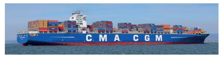
he Maltese-flagged ship is 42.87 metres wide and has a nominal container capacity of 9658 TEU and 700 reefer points, according to its operator, CMA CGM. The vessel is on the A3 Central Express service, which calls Kaohsiung, Xiamen, Shanghai, Ningbo, Sydney, Melbourne and Brisbane before heading back to Kaohsiung to start the loop again.
